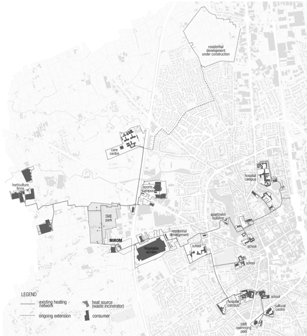
Figure 2.2. The existing district heating network in Roeselare, including the waste incinerator and diverse customers. Source: elaborated by author based on data from Mirom, Stad Roeselare, and GRB, Agiv.
