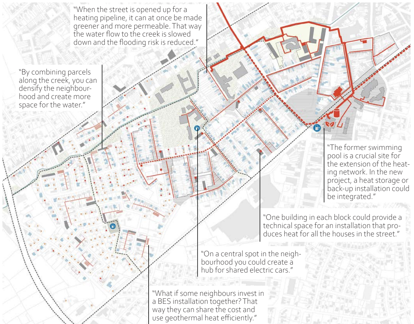
Figure A.32. Zoom 3: Groenpark, De Spil: collection of design workshop ideas for a neighbourhood energy strategy. Source: author based on workshop.
